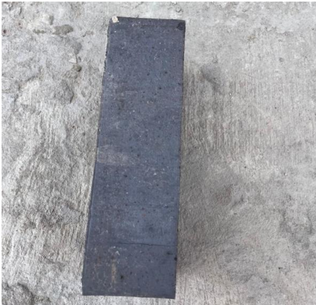
Plinth bricks-Staffordshire blue bricks
